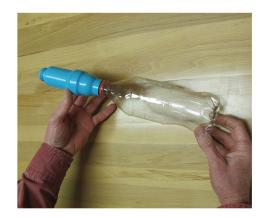
3. Connect syringe or plastic bottle to housing and flush with FILTERED water until discharge is clear.
