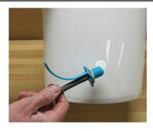
2. Insert bucket connector by placing one washer on either side of hole.
