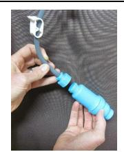
Remove filter housing from tube.
