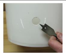
1. Use the hand held drill to drill a hole in the bucket. Place hole 3 inches from bottom of bucket to allow for sediment accumulation. The recipients should drill their own bucket and assemble their own filter as this will increase their sense of ownership.
