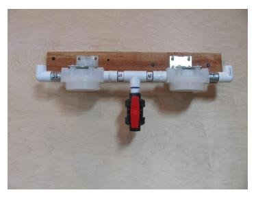
Bolt Filter Mount Assembly to wall with toggle bolts provided. Assembly should be a minimum of 75mm or 30 inches above the floor in order to remove filter housings at a later date. Check to make sure there is room for the remainder of the unit to the left or right of the Filter Mount Assembly.
