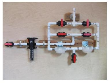
Cement the Prefilter to the Valve Control Unit using the Water Line Connector. Cement the Supply Line Control to the Prefilter. Place metal straps over the PVC line as needed support. Use screws provided.
